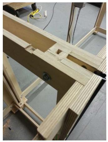
**15. Take the time to verify the levelling between** the two structure modules and make the final adjustment. You should place the structure where it is meant to be for the exhibition because **you won't be able to move the piece later on**.
