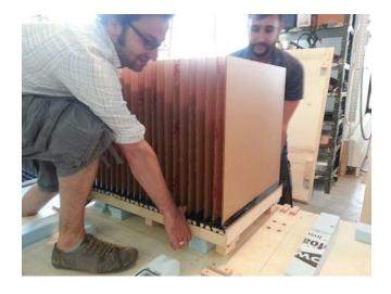
**22.** Grip hardly the stainless steel tubes and lift the module while keeping it parallel to the ground.
