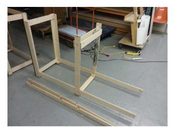
7. Install the two last trusts (the ones with the channels)
