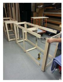
**9.** Make sure that all the screws are in place (2 screws per joints).
