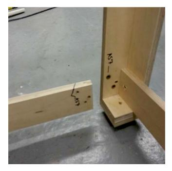
**6.** When the bottom trusts are installed you can get the middle set of legs in place.
