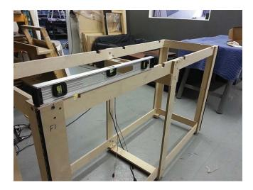
**14.** Install the 4 wood spacers. There are marks on them so you can find the right place to install them. **HINT** : longer screws need to be with the spacers of the bottom, shorter screws at the top (if not, the longer screws will prevent the acrylic module to be properly placed).
