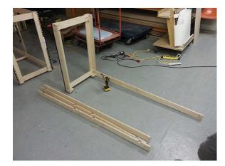
**5.** All the joints are identified with letters and numbers to easily match the parts together.
