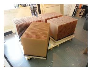
**21.** Use the two stainless steel tubes to get a good grip under the LED modules. <u>You need to be at least two persons</u> to lift a module. **HINT** : There are channels under the LED module, so you only have to slide the tube into them.
