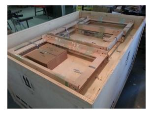
**4.** Start the assembly from the bottom part. Each structure contain : 3 Sets of legs and 4 trusts. **HINT** : There is two structures to build so you should split the parts to be sure you don't make mistake while making the assembly.
